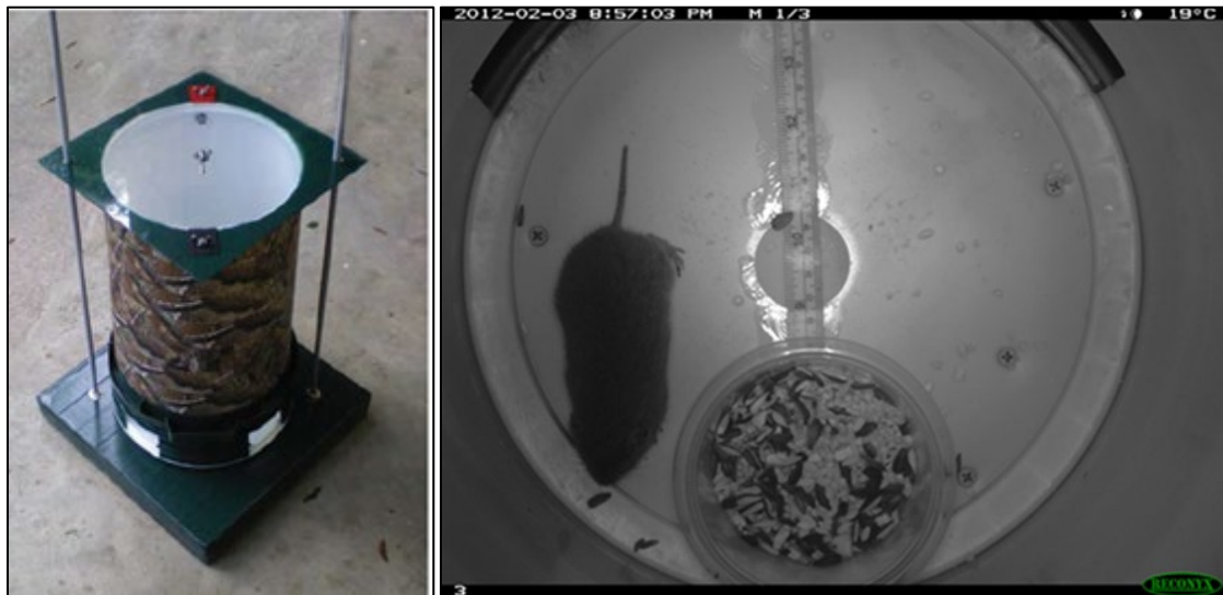
Figure 2-3. Left: Floating camera trap for small mammals (McCleery et al. 2014, p. 888). Right: FSMV image capture in the bucket trap.
