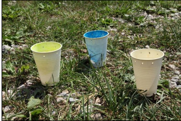
Figure 3. Propylene glycol cup trap (12-oz), painted in fluorescent blue, fluorescent yellow, and white.
