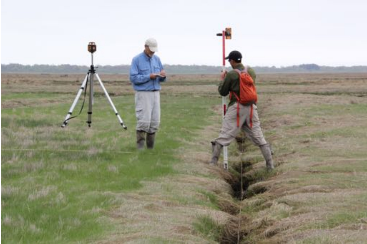
Figure 18. Surveying marsh surface, ditch edge and bottom elevations along perpendicular transects in Nelson's Island marsh.
