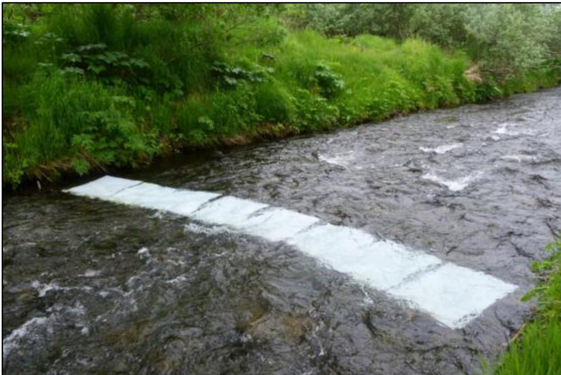
Figure 3. White substrate panels that highlight passing salmon. They are secured to a chain that spans the stream and is anchored to the bank with rebar or T-posts.
