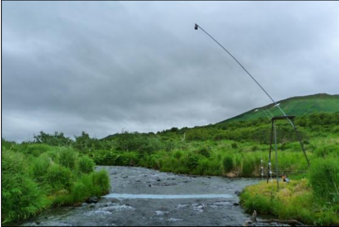
Figure 2. Camera system at Moraine Creek. Note steel tripod and white contrast panels.
