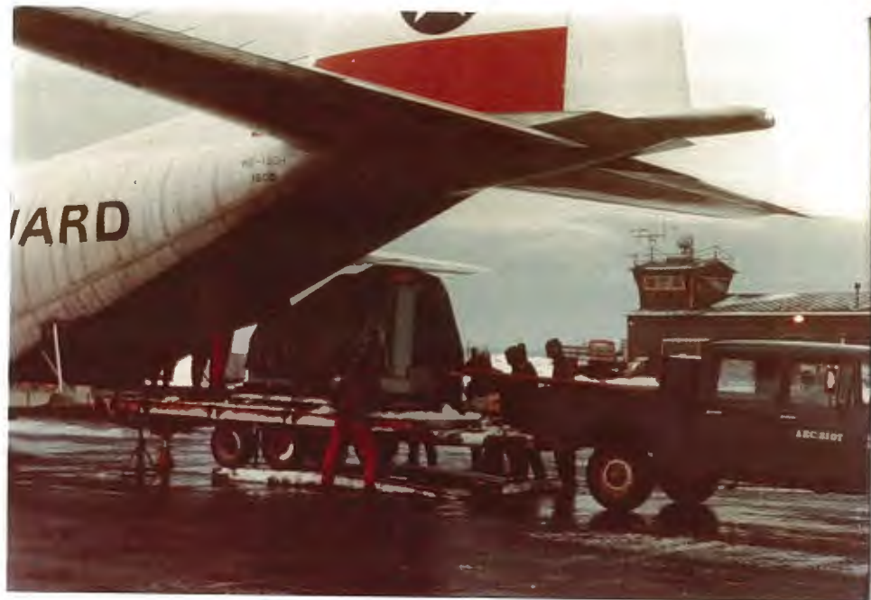
The YACC crew at Amchitka unloading a new 100 KW generator from a U.S. Coast Guard C-130. Schulmeister
