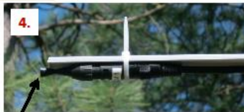
Horn should extend approx ¼ inch past angle aluminum
